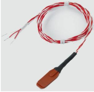
Self adhesive bendable Pt100 sensor. Silicon patch size 35x13x2mm. Fast response by use of self-adhesive aluminium contact foil to attach to the surface. Temperature range: up to 170°C. Accuracy to DIN IEC 60751 class B, optional class A. Single sensor. Sensor is standard 3-wire connected. IP54 sealed. Twisted PTFE wires. Standard wire length 4 meter. Good chemical resistance. Response time 2 sec. Maximum peak temperature 220°C
