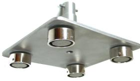
Powerful magnet mounting plate for indoor and outdoor usage, equipped with four high temperature magnets, each 2500 Oe. (200 kA/m). Maximum temperature 300 °C Stainless steel SS316 Mounting plate, 100x100mm has a bayonet mount for installation of spring-loaded sensors with a diameter up to 6mm. Bajonet connection for 1 or 2 slots and available in 2 different diameters
