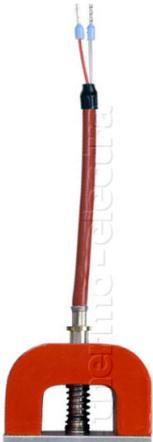
Magnetic surface Pt100 sensor, magnet dimensions 39x26x25mm (LxBxH), Magnetic strength 90 N. Accuracy to DIN IEC 60751 class B, optional class A. Sensor is standard 3-wire connected. Silicone cable with flexible conductors, standard cable length 4 meter. Good chemical resistance. Can be used on feretic surfaces. Maximum temperature at tip 250°C. Spring loaded sensitive contact tip. Thermal conductive paste on rough surfaces recommended. Options: ATEX Exe or Exi version
