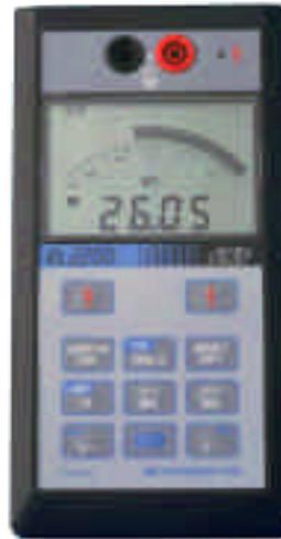
The RL2200 is particularly suited to maintenance, verification and reception of telephone lines, and more generally of all low voltage cables. Its unique dual display offers both digital readings, for high accuracy measurements, and analogue readings to «feel» measurements tendency and monitor threshold limits.
