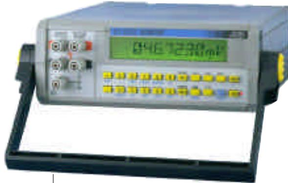
SN 8310 is a standard dc voltage and current source. It will supply voltages from 100 nV to 110 V and currents from 1 nA to 110 mA with an accuracy of better than 0,002% (20 ppm).
