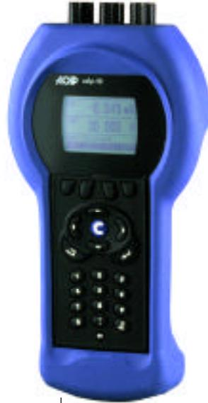
The calibrator CALYS 10 is designed to meet all the growing requirements of the calibration and maintenance departments, either on site or in laboratories. Built in with a protective housing and with a quick charge battery, it can control, verify and calibrate all the instruments entering in the process in industrial areas.
