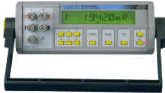
The OM22 micro-ohmmeter is used for four-wire resistance measurement of very low values (with a resolution of 0.1  $\mu\Omega$ ) up to 20 k $\Omega$ , with an excellent accuracy
