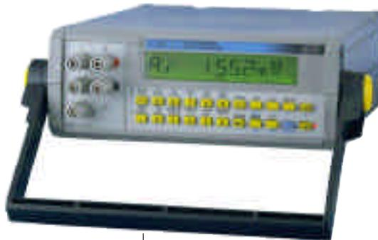
OM21 micro-ohmmeter is used for four-wire resistance measurement of very low values (with a resolution of 0.1  $\mu\Omega$ ) up to 20 k $\Omega$ , with an excellent accuracy.
